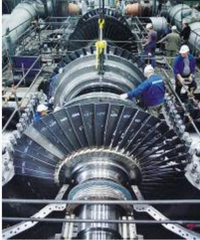
Figure 3. Steam turbine in a power plant.<sup>[5]</sup>
