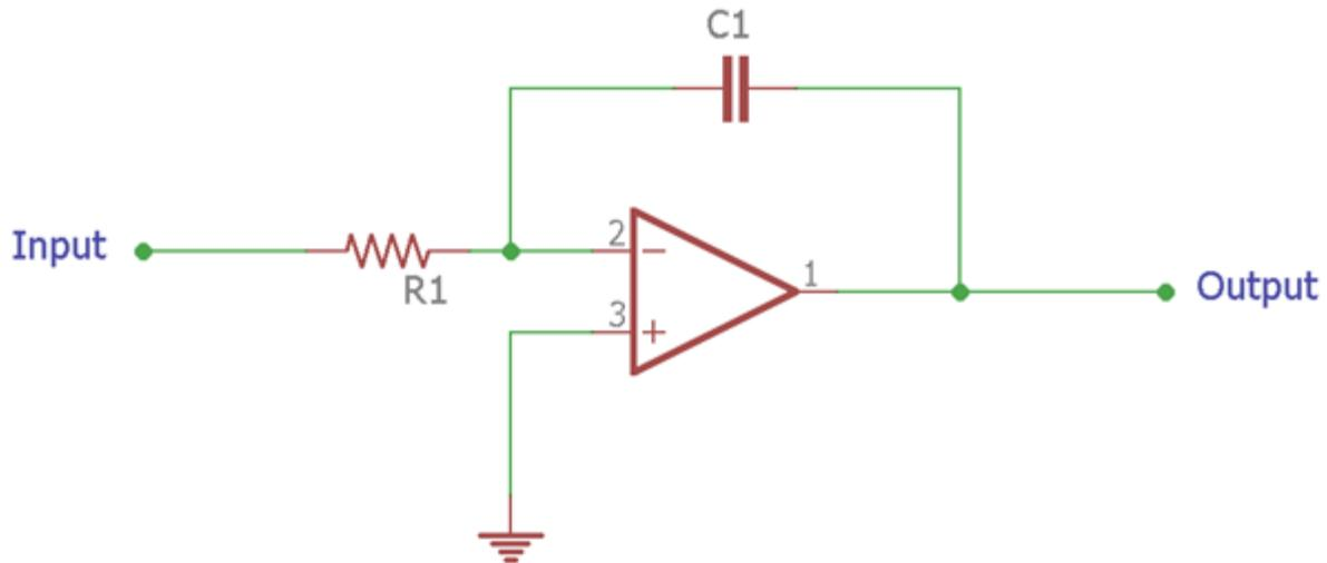
The construction of simple Integrator circuit using op-amp requires two passive components and one active component. The two passive components are resistor and capacitor. The Resistor and the Capacitor form a first-order low pass filter across the active component Op-Amp. Integrator circuit is exactly opposite of Op-amp differentiator circuit.
