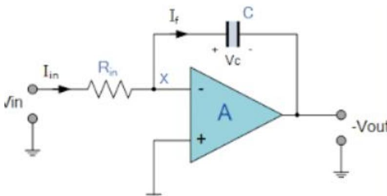
**A simple Op-amp configuration consists of two resistors, which creates a feedback path. In the case of Integrator amplifier, the feedback resistor is changed with a capacitor. The resistor R1 and capacitor C1 is connected across the amplifier. The amplifier is in Inverting configuration.**
