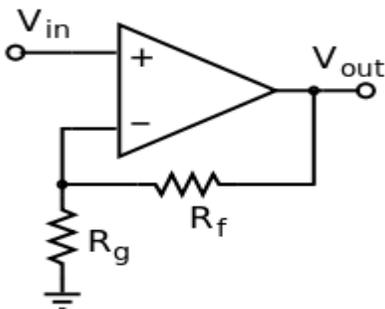
If the feedback network is made of components with values small relative to the op-amp's input impedance, the value of the op-amp's open-loop response  $A_{OL}$  does not seriously affect the circuit's performance. The response
