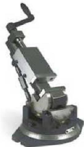
The universal vise allows the operator to tilt the workpiece 90 degrees in the vertical plane as well as swivel it 360 degrees in the horizontal plane.
