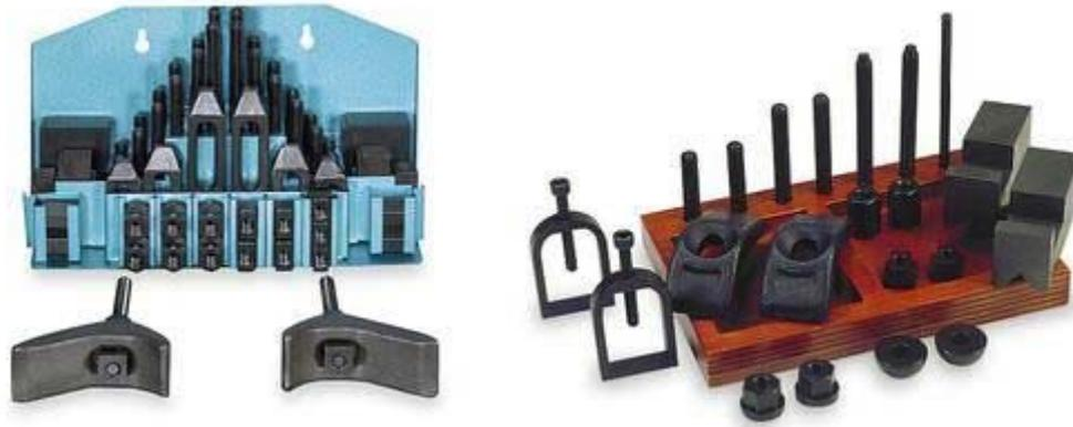
Figure 12: Clamping Sets
